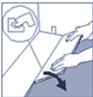
Fig 3. Tilt angle the panel down. During the angle process make sure the panels are tight against each other. Afterwards press down or slightly tap down at the short end or long edge of the installed plank till its flat. No major force is or required.
